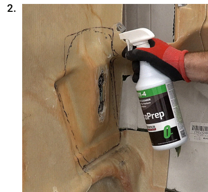
2. Clean the damaged area of the hood. Dry completely.
