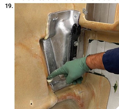
Using a gloved finger, smooth any squeeze-out. Let cure 24 hours before installing the hood onto the truck.
