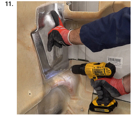
Carefully drill a 1/4" hole through the hood, using gentle pressure and high speed to prevent tear-out on the outside of the hood.
