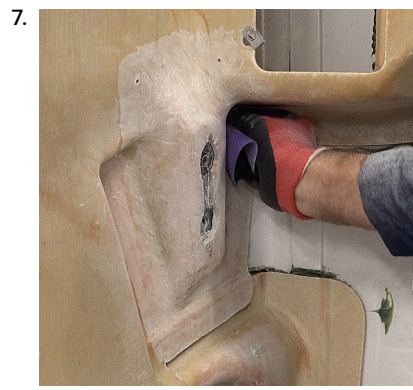
7. Hand sand any areas missed using the Roloc® disc on both the hood and aluminum casting.
