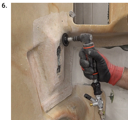
6. Sand the hood with the Roloc® disc.
