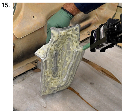
Apply a very generous amount of 2510 PlastiFix to the back of the casting.
