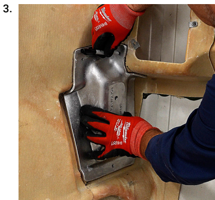
3. Place the casting over damaged area and trace the casting. Mark all holes in the casting flange
