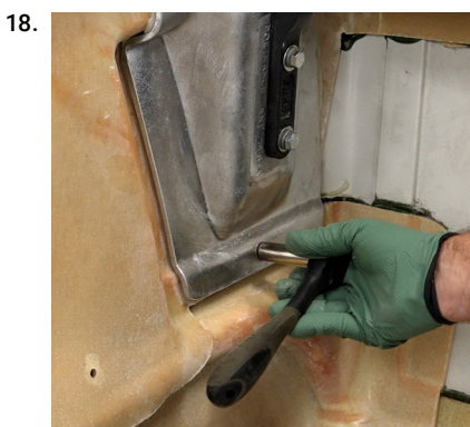
Snug the nut on the elevator bolt. Put threadlocker or a dab of 2510 on the threads to keep it from loosening.
