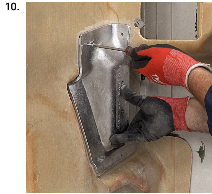
Loosely screw the casting in place to help keep it aligned while drilling the 1/4" hole for the elevator bolt.
